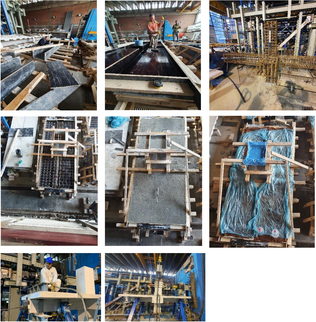
Figure 2.20. Construction stages for PTI-4-50
