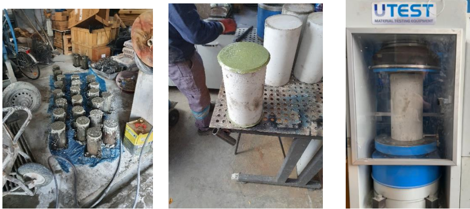
Figure 2.9. Concrete compression test
