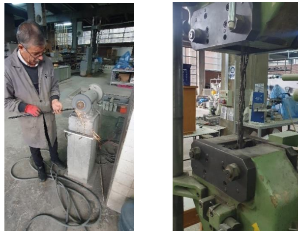
Figure 2.12. Direct tension tests for prestressing steel
