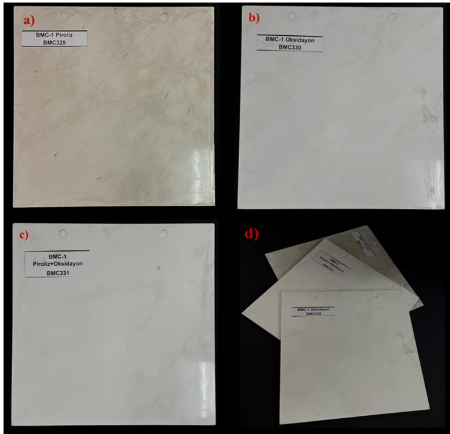
Figure 4.21. Recycled BMC composite plates. a) Pyrolysis, b) Oxidation, c) PO, d) All together
