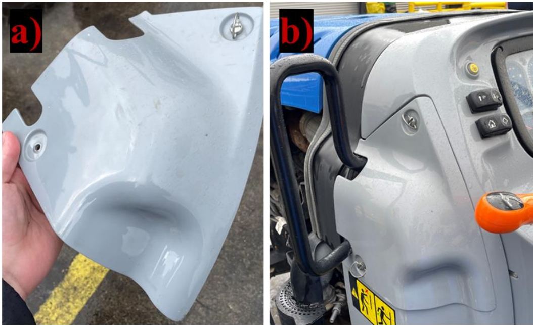
Figure 4.37. Tractor component produced with recycled BMC. a) by itself, b) on the tractor
