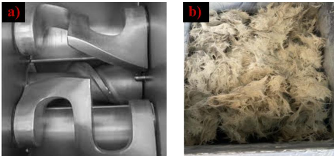
Figure 3.9. Dough mixer used in composite production. a) Z-type blades, b) Dough before mixing
