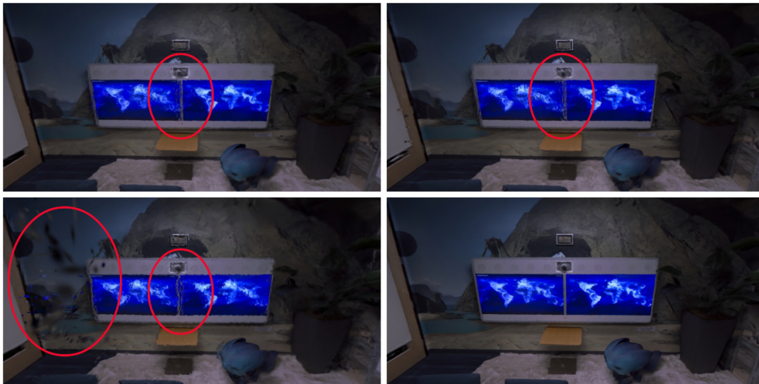
Figure 6.3: Qualitative Results for Learning Rate Decay Ablation Study . The four cases examined in Table 6.7 are presented in the figure. The results include constant learning rates of 1.6 \times 10^{-4} at the top-left , 5 \times 10^{-5} at the top-right , 1.6 \times 10^{-6} at the bottom-left , and the decaying 1.6 \times 10^{-4} learning rate at the bottom-right as a reference. The figure is adapted from [10]
