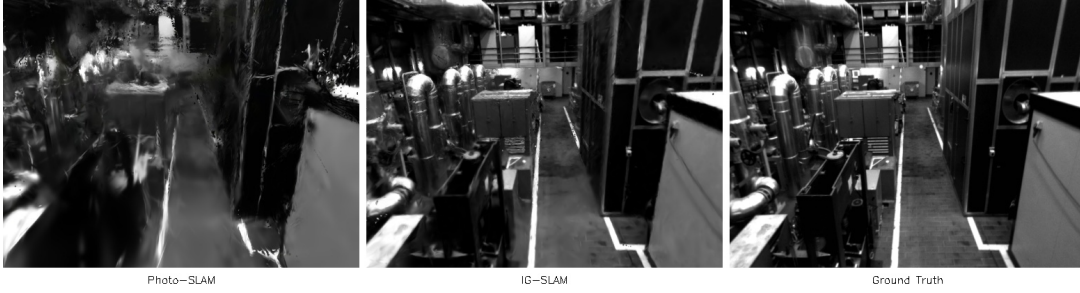
Figure 6.1: Qualitative rendering results from Photo-SLAM [47] and IG-SLAM. The visual quality of the methods is compared on the large-scale EuRoC dataset [57].
