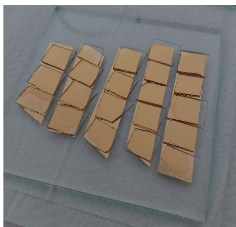
Figure 2.4. Glass wafers adhered to mica-gold strips, prepared for subsequent sandwiching between two glass pieces, and curing with UV light.
