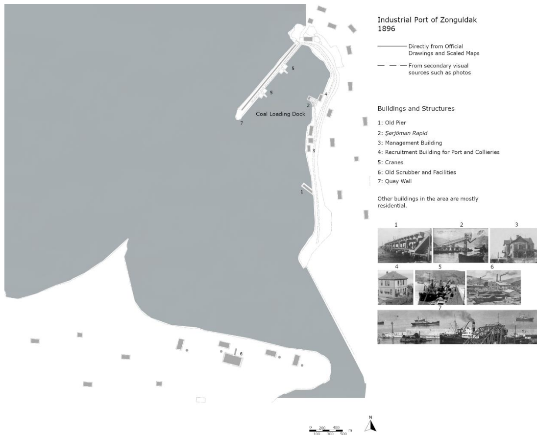
Figure 89: Industrial Port of Zonguldak, First Period, produced by the author, base drawing from Zonguldak Municipality, base image from General Directorate for Mapping
