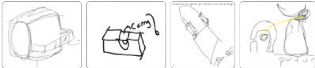
Figure 4.59 Sketch examples for handle solutions. Left. Edgy and rubber strap. Second from left: Flat strap with sculpted body. Third from left: The body of the speaker turns to the handle to wrap on a bag strap. Right: Clip to hang.
