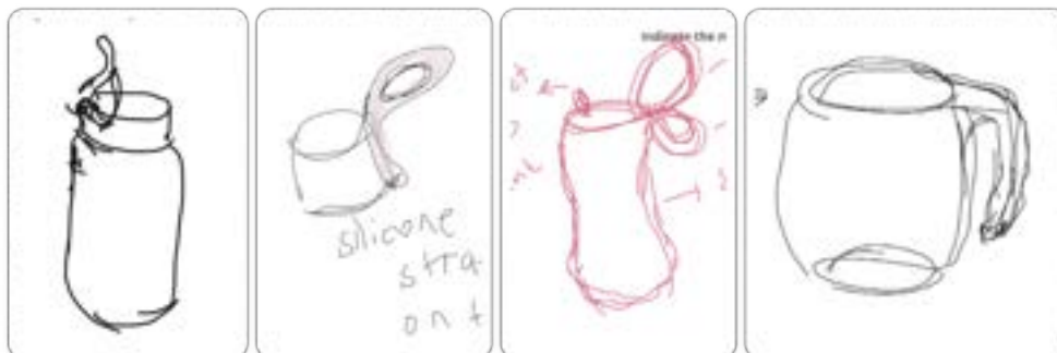
Figure 4.27 Sketch examples for handle solutions. Left: Hoop-formed handles. Two in the middle: Loop-formed handles. Right: Open-ended handle at one side.
