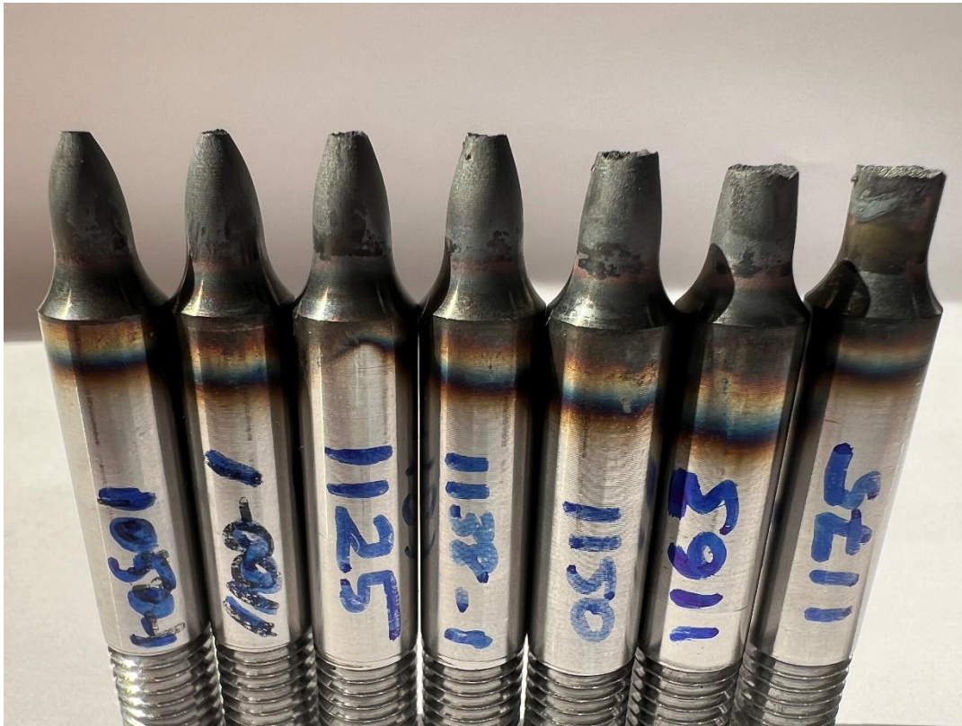
Figure 4.18. Specimens after hot tensile tests at various temperatures
