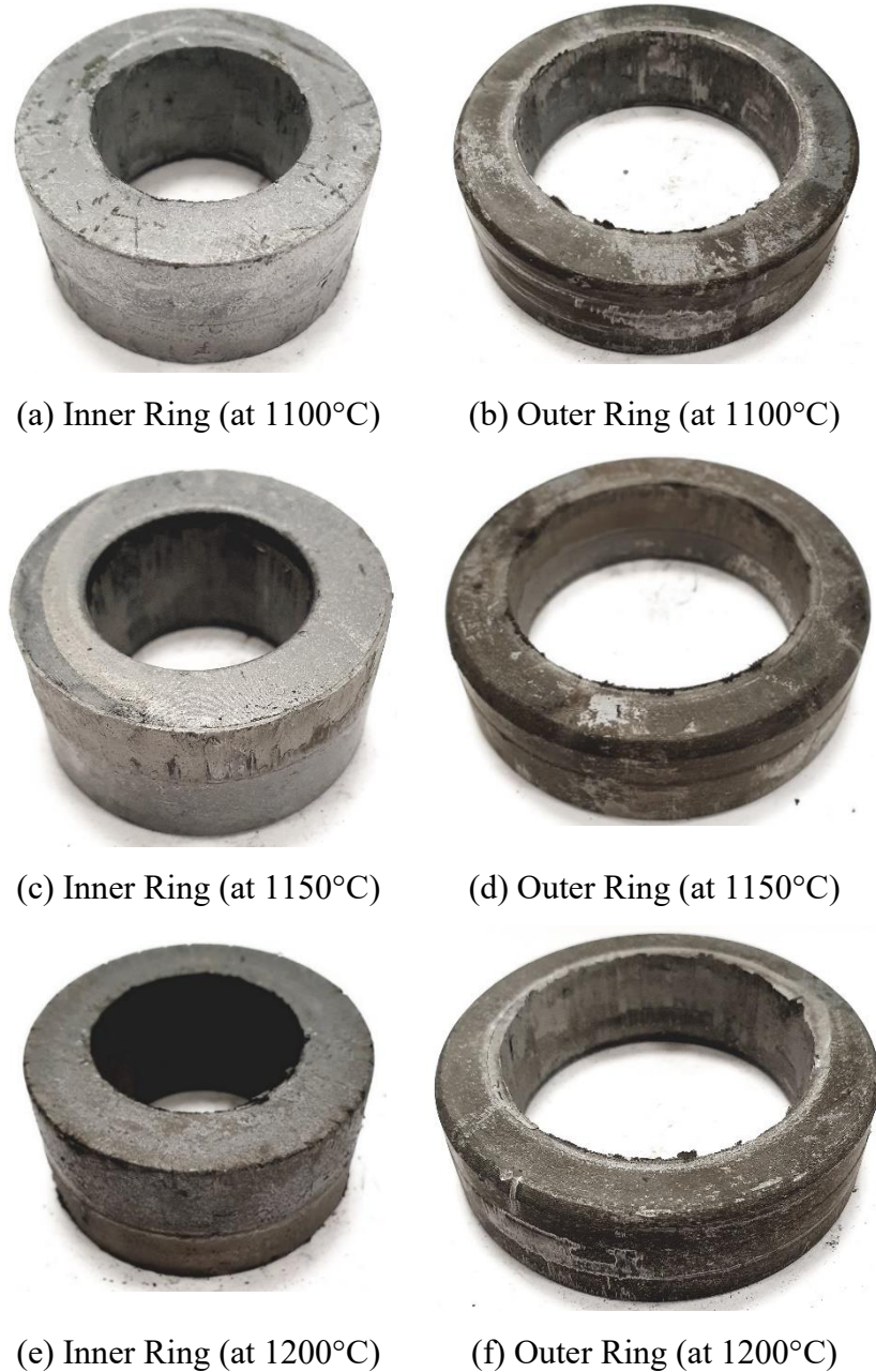
Figure 5.12. Inner and outer rings after hot forging experiments at ORS with 0.4 mm die clearance
