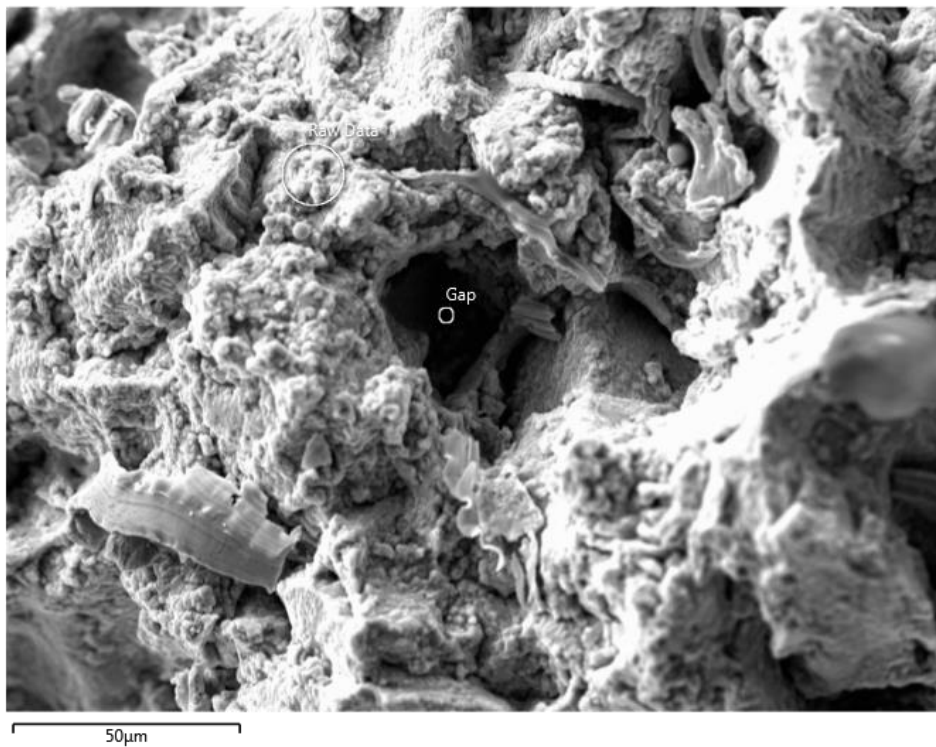
Figure 4.34. Dimple on the fracture surface after tensile test at 1150°C
