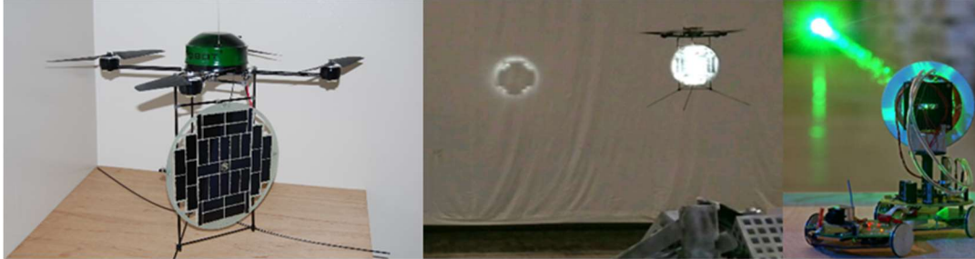
Figure 2.3. Multicopter powered by laser at Kinki University in 2008 (on the left and middle) [20], laser-powered rover developed by EADS (on the right) [21]
