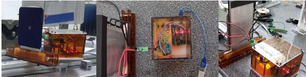
Figure A.2. Images of the measurement system connected to an IBC cell while measurement
