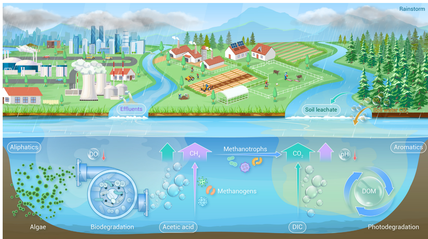
Figure 1. Rainstorm-induced organic matter inputs drive carbon emissions from inland waters Shown is a schematic of how a rainstorm event increases input of terrestrial dissolved organic matter (DOM), alters water chemistry, and promotes the outgassing of carbon dioxide ( \text{CO}_2 ) and methane ( \text{CH}_4 ) in downstream lake ecosystems, particularly in inflow areas. DO, dissolved oxygen; DIC, dissolved inorganic carbon.
