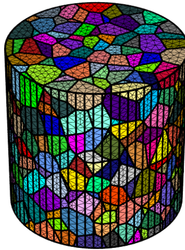
Figure 4.2-1 RVE created by Neper to be used in CPFEM simulation
