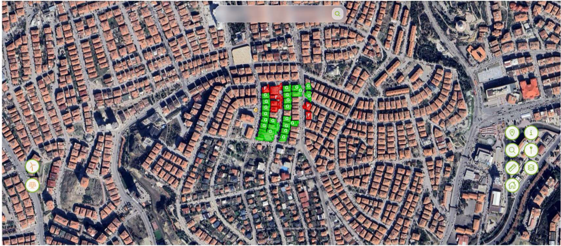
Figure 5 - Prototype web application interface demonstrating the visualization of detected roof polygons and predicted roof-type classes layers on an interactive map.
