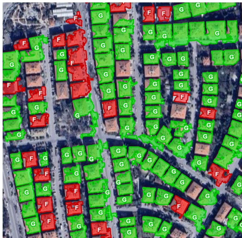
Figure 10 - Final roof inventory visualization after filtering out polygons classified as "Bugs", highlighting the role of the classification stage as an implicit noise-removal mechanism.
