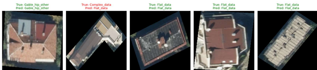
Figure 4 - Representative roof-type classification results on test samples, comparing ground-truth labels with model predictions.
