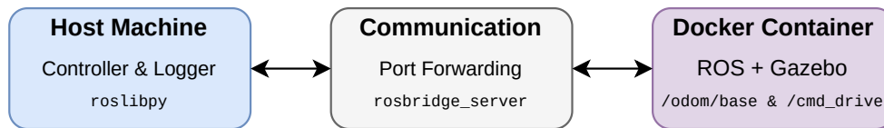
Figure 4.2: Host–Docker communication diagram for ROS-based simulation control.
