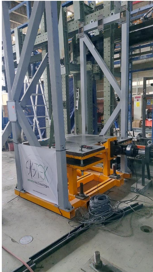
Figure 5.3 Shaking table which installed in the laboratory
