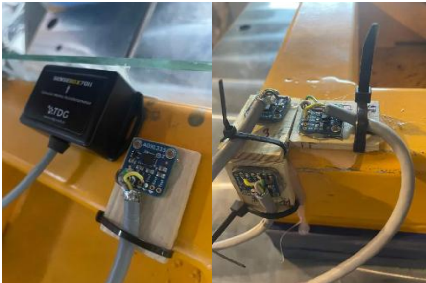
Figure 5.8 Mounting the accelerometers manufactured in the laboratory side by side to compare the measurements of branded accelerometers.
