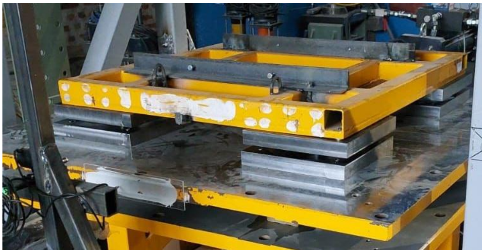
Figure 5.5 The installed isolated slab in the laboratory
