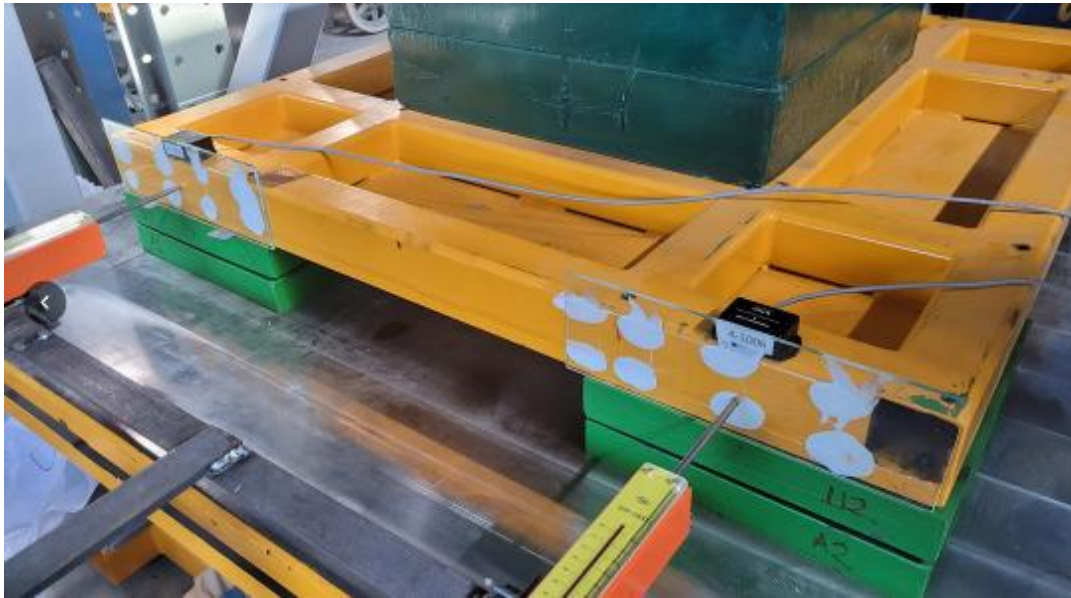
Figure 5.10 Potentiometers and accelerometers are placed on both corners of the isolated slab for acceleration data verification.
