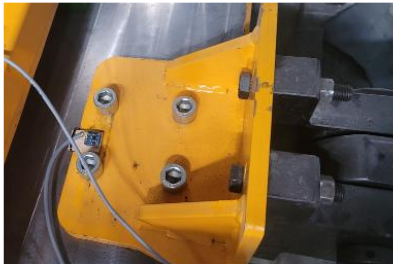
Figure 5.9 The accelerometer fixed directly on the hydraulic actuator connecting piece on the direction of excitation.
