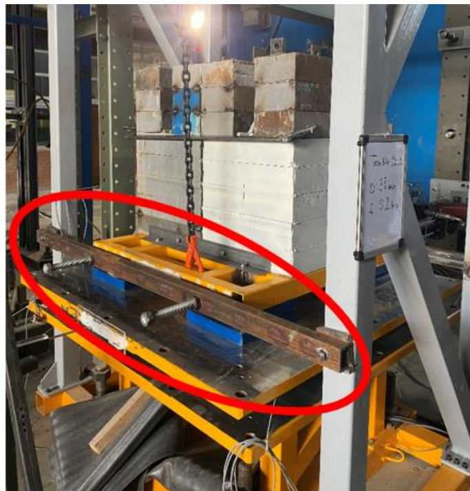
Figure 6.6 The modified test setup for obtaining the force-deformation curves of floor isolators (the element that prevents horizontal movement and allows vertical movement is enclosed in a red circle).
