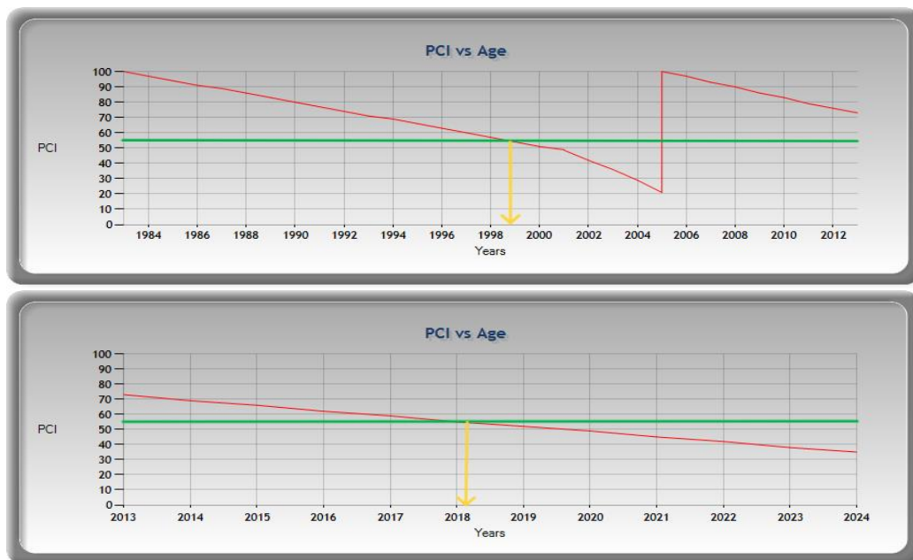
Figure 4.14 Apron alpha condition analysis (1983-2024)
