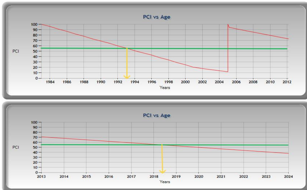
Figure 4.12 Runway End28 section condition analysis (1983-2024)
