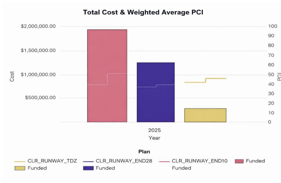
Figure 4.29 Runway sections CLR M&R cost for Year 1
