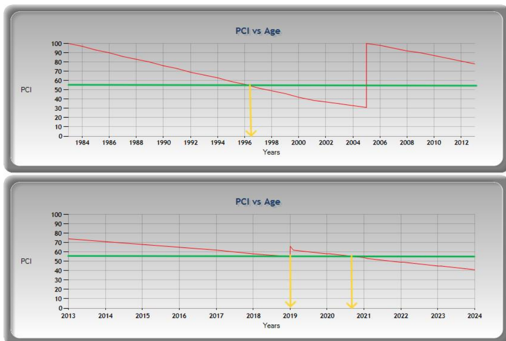
Figure 4.13 Runway Touchdown zone condition analysis (1983-2024)
