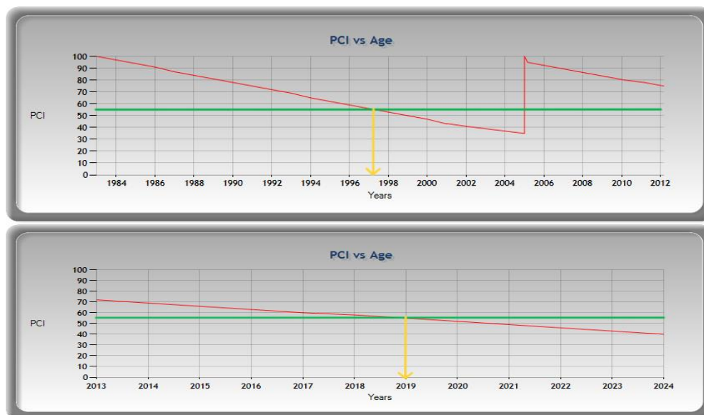
Figure 4.11 Runway End10 section condition analysis (1983-2024)
