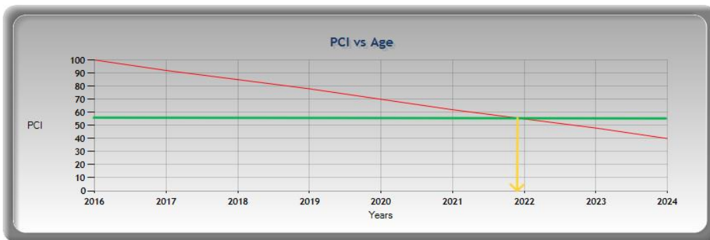
Figure 4.15 Apron Bravo condition analysis (2016-2024)
