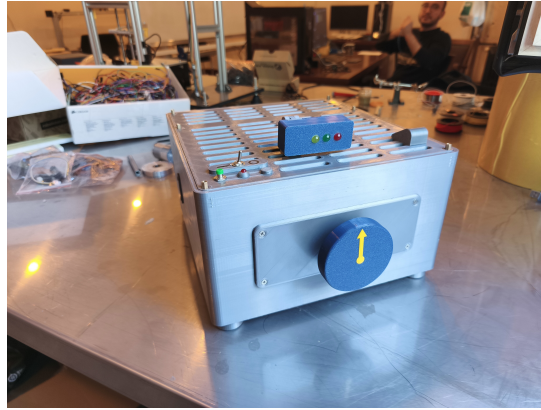
Figure 2: The custom 1-DOF haptic device used in the experiment.
