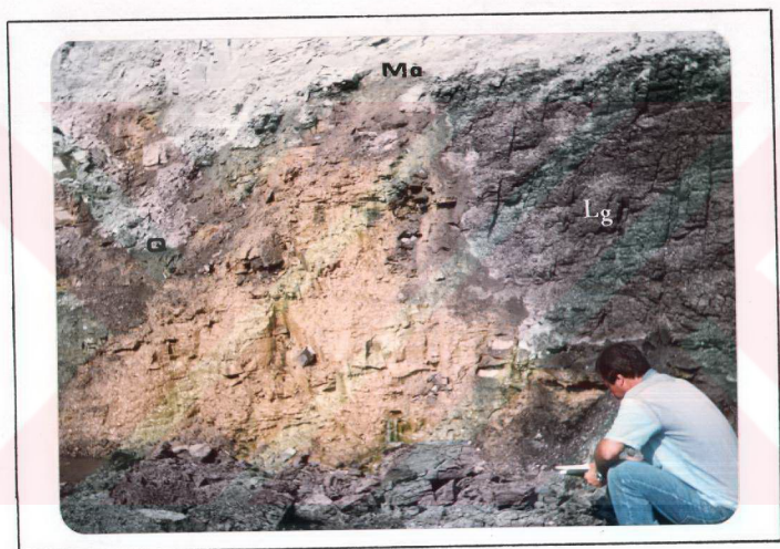
Figure 33: Seepage from the coal seam and compact marl/coal seam boundary at the new higwall face - south of ninth slice (Lg: Lignite; Ma: Marl; Plate 3-Photo. No.16).
