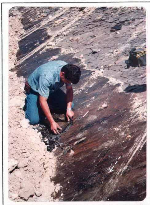
Figure 62: Plane failure on footwall material-slide 8: (A) instability plan and structural features; (B) sliding surface and linear traces parallel to movement direction (Plate 3-Photo. No.24); (C) kinematic check of the failure.
