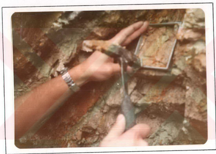
Figure 41: Undisturbed and oriented sampling from a fault gouge using metal specimen cutter (Plate 3-Photo. No.22).
