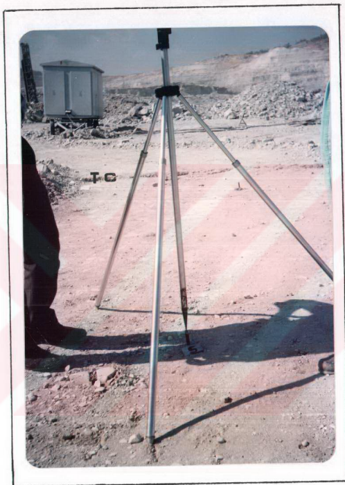
Figure 34: A monitoring target consisting of reflector prism, tripod and labeled steel bar for the monitoring of surface displacements (TC: Tension crack; Plate 3-Photo. No.17).
