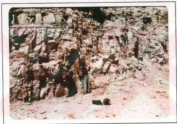
Figure 23: View showing discontinuity survey conducted on compact marls and joint pattern developed in this rock unit (Plate 3-Photo No. 13).
