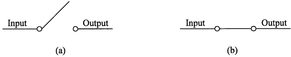
Figure 2.10: Schematics of a simple switch. (a) The switch is off. Input and output are disconnected. (b) The switch is on. Input and output are connected.
