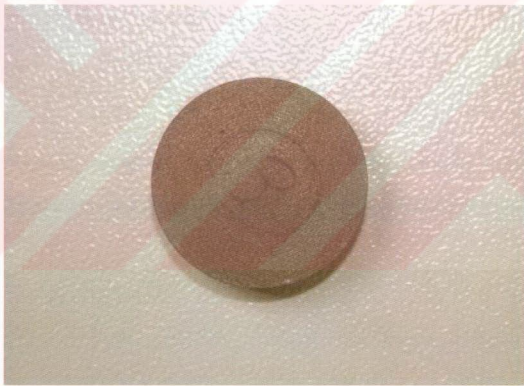
Figure 4.19. A cylindrical sintered compact before hot rolling
