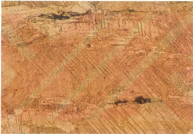
Figure 4.21. The optical micrograph of Cu-12 w % Al, hot rolled after sintering at 950°C X150
