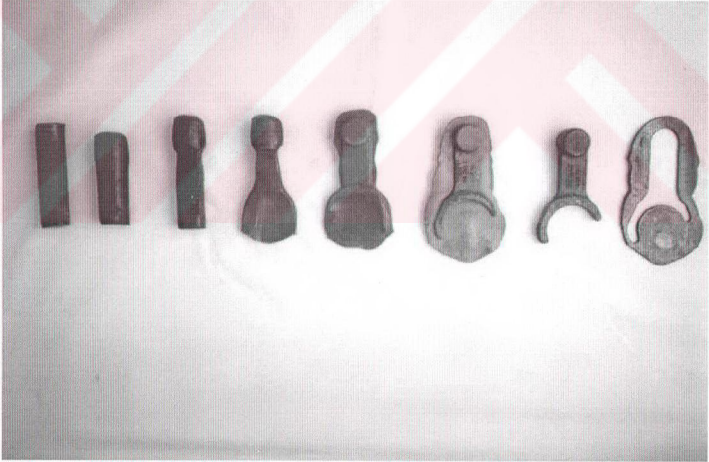
Figure 5.2 Manufacturing steps of the forging 198-290.2
