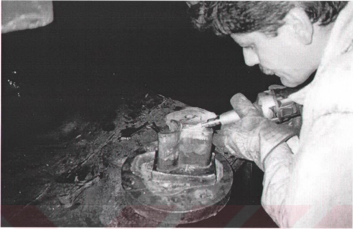
Figure 5.10 Trimming dies needed frequent maintenance
