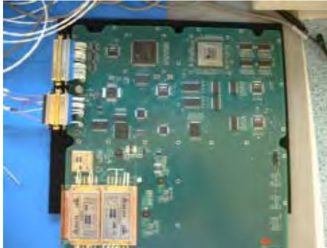
Figure 4.1 Photograph of GEZGIN, the image compression system which is designed as a payload for a LEO micro-satellite, BILSAT-1. (The photograph is provided with the courtesy of TÜBİTAK-BİLTEN).
