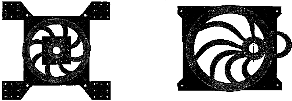
Figure 3.13 Multidirectional EP Device in Neutral Position and at Maximum Deflection
