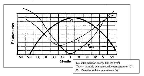
Figure 2.3 Heat requirement in a greenhouse over a typical year in Gevgelia, Rep. Of Macedonia (Popovski, 1984)
