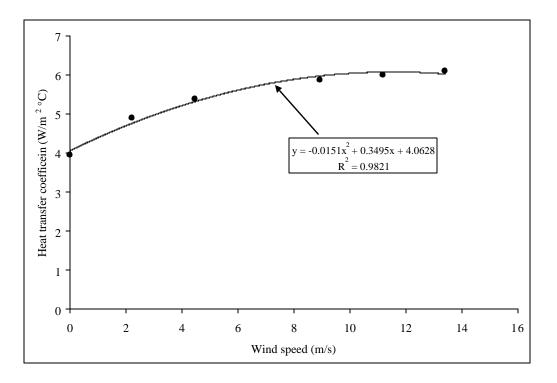
Figure A.1 Heat transfer coefficient for fiberglass as function of wind speed.
