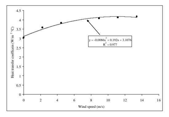
Figure A.3 Heat transfer coefficient for doublepoly as function of wind speed.
