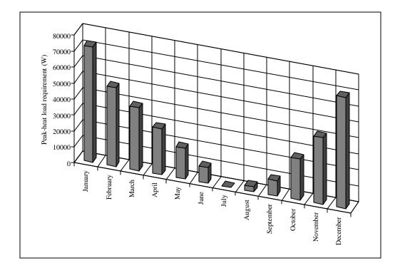
Figure 4.13 Monthly peak-heat requirements for glass at 12 °C indoor temperature.
