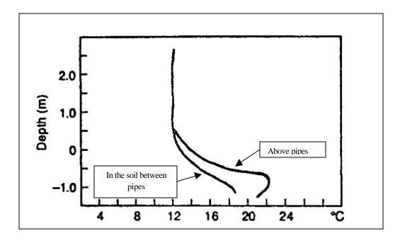
Figure 2.5 Vertical temperature profiles in a greenhouse with soil heating (Dickson and Fanelli, 1995).
