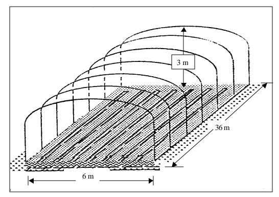
Figure 4.11 Shape and size of a greenhouse.
