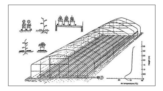
Figure 2.7 Heating systems on soil surface or on the benches (Dickson and Fanelli, 1995).
