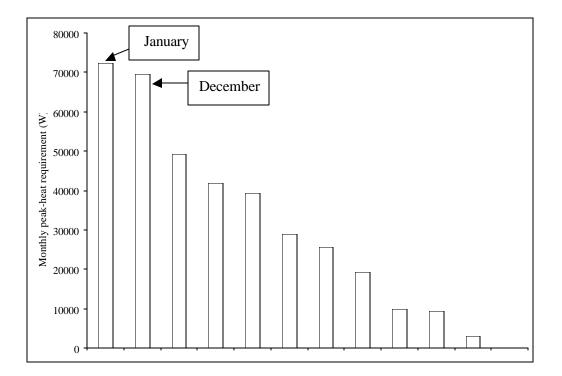
Figure 4.15 Sorted monthly peak heat loads calculated for glass as glazing material at 12 °C indoor temperature.
