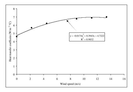
Figure A.2 Heat transfer coefficient for singlepoly as function of wind speed.
