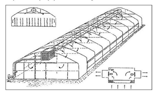
Figure 2.9 Fan-coil air heating system (Dickson and Fanelli, 1995).
