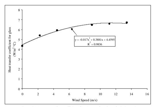
Figure 2.11 Heat transfer coefficient for glass as function of wind speed.
