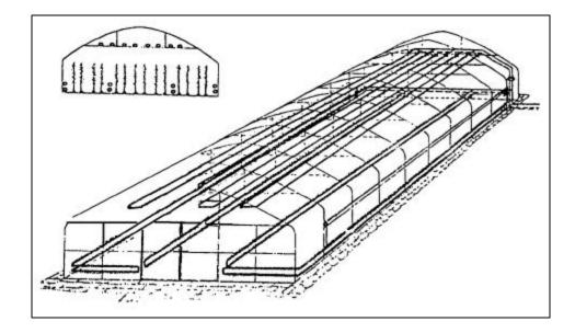
Figure 2.8 Aerial pipe heating installations (Dickson and Fanelli, 1995).
