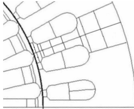
Figure 4.3 The regions assumed to exist in one tooth pitch of the stator core
