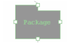
Figure A.10. COSEML Figure Represents Design Pattern Package (when design pattern is used in detailed mode)
