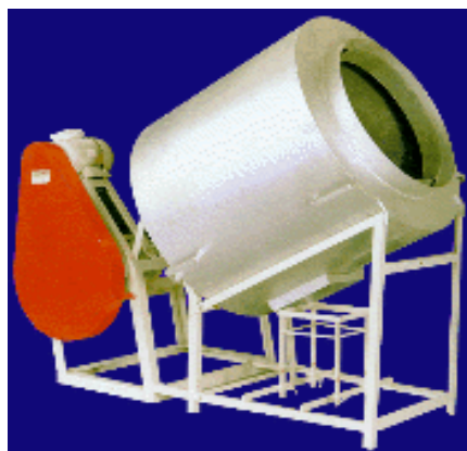
Figure 6: Roaster with rotating boiler (Gürmaksan, 2003)
