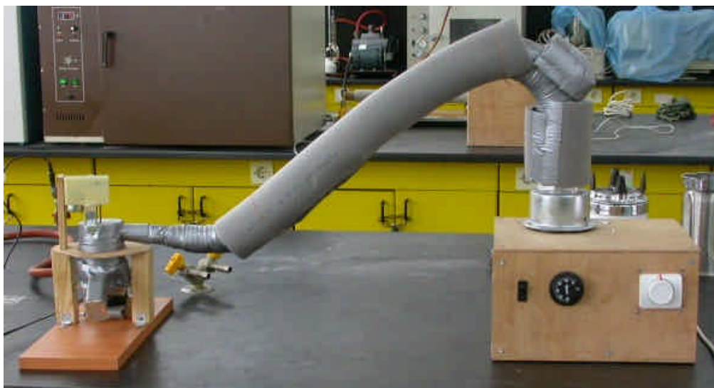
Figure B.8: Photo of hull separator with air source
