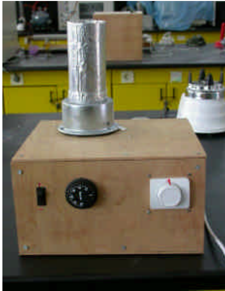
Figure B.3: Photo of fluidized bed dryer
