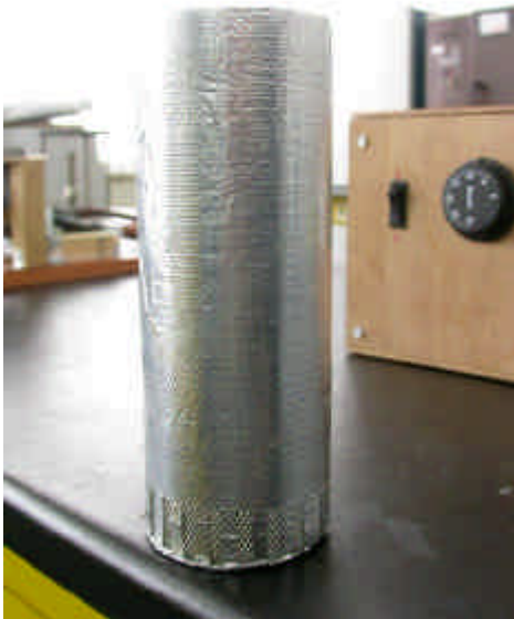
Figure B.4: Photo of fluidized bed column
