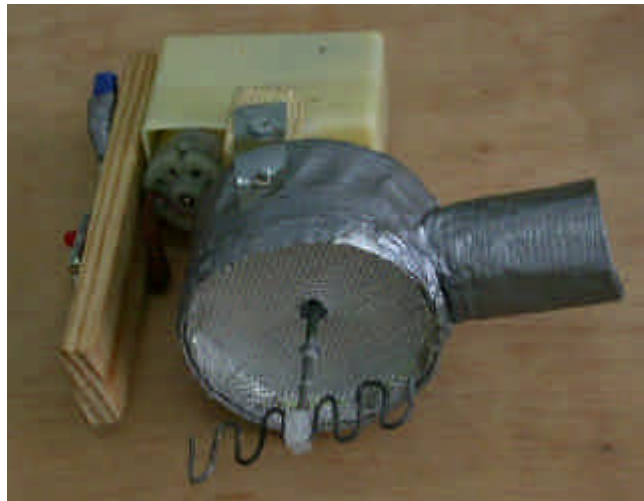
Figure B.7: Photo of air distributor and agitator paddle of hull separator
