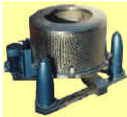
Figure 5: Sesame centrifuge (Gümüs, 2003)
