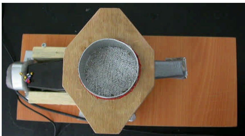
Figure B.6: Photo of fixed vessel and sieving equipment at the bottom side of hull separator
