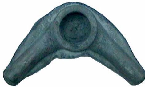
Figure 5.9 – Preform after Blocking Operation
