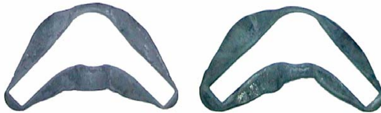
Figure 5.11 – Two Different Flash Formation Occur at Finishing Operation
