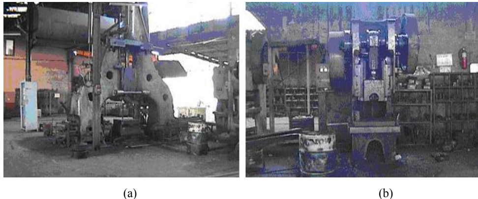
Figure 4.3 – (a) “5000 kgm” Drop Hammer; (b) “200 tonf” Mechanical Press
