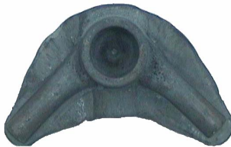
Figure 5.10 – Part after Finishing Operation
