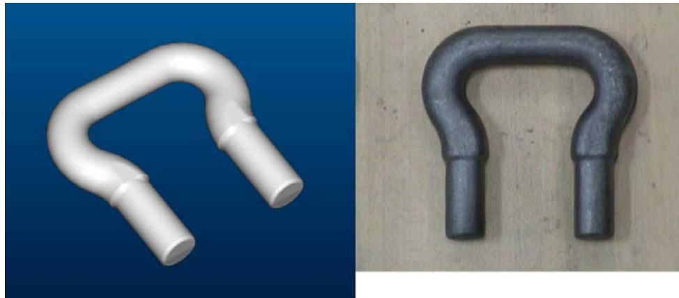
Figure 4.1 – Chain Bracket (DIN 745 – 63)
