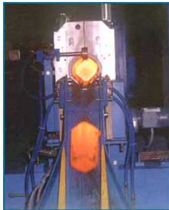
Figure 5.4 – “970 kW” Induction Furnace of “4000 tonf” Press Line
