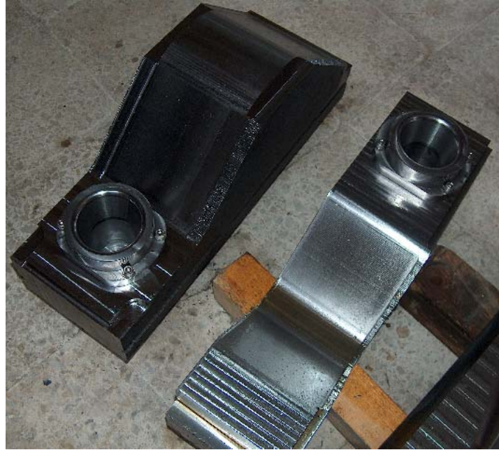
Figure 5.36 – Manufactured Dies of 1 st and 3 rd Preform Operations (Upsetting and Bending)
