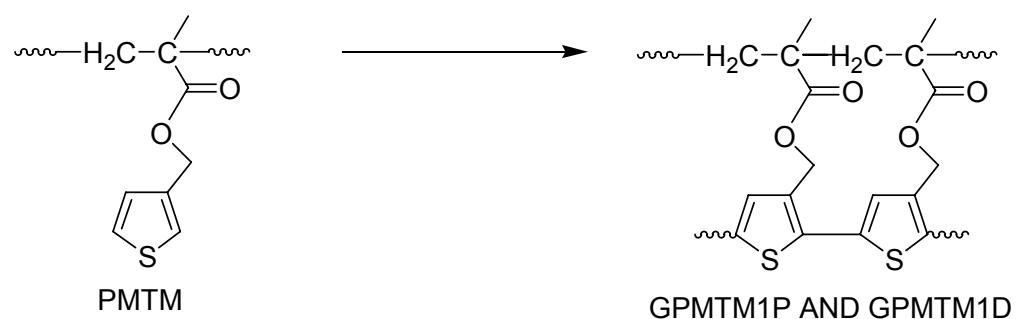
Figure 3.3. Galvanostatic polymerization route
