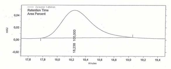
Figure 31. The HPLC-Chromatogram of (+)-54b
