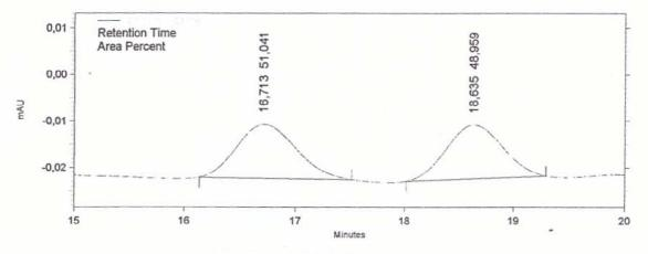
Figure 36. The HPLC-Chromatogram of the Racemic 2-Hydroxycyclopentanone
