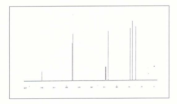
Figure 23. <sup>13</sup>C-NMR Spectrum of (-)-7-Oxabicyclo[3.2.1]oct-2-en-6-one (20)
