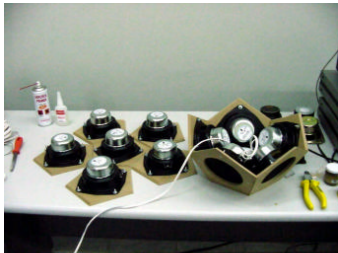
Figure 5.27 Constructional Details of the Omni-directional Source
