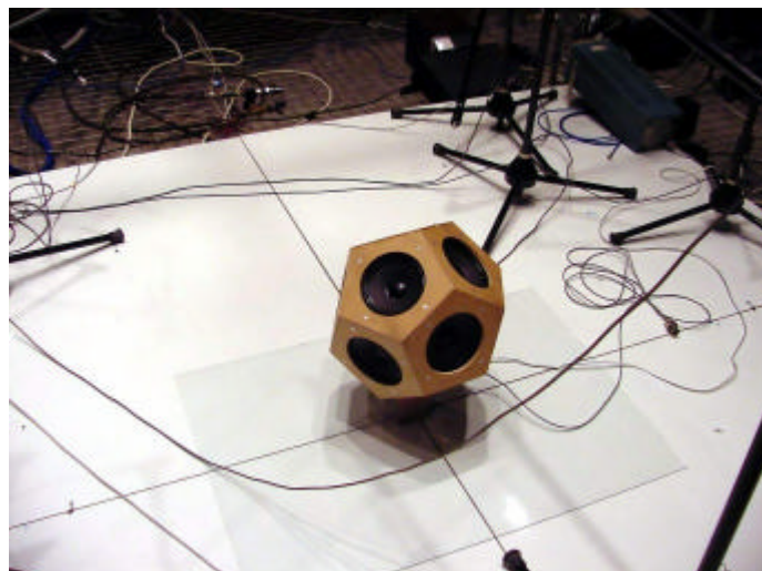
Figure 5.28 Omni-directional Source as Finished
