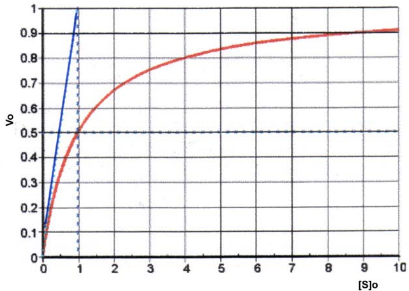
Figure 1.11 A normalized plot of the initial rate ( v_0 ) against initial substrate concentration ( [S]_0 ) for a reaction obeying the Michaelis-Menten kinetics (equation 1.8).
