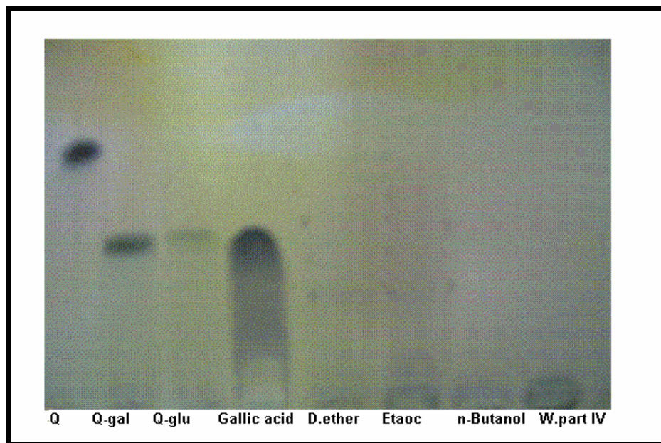
Figure 19: TLC data of for all organic fractions of Punica granatum (pomegranate), visualization with \text{FeCl}_3 Q: Quercetin, Q-Gal: Quercetin-3-galactoside, Q-Glu: Quercetin-3-glucoside
