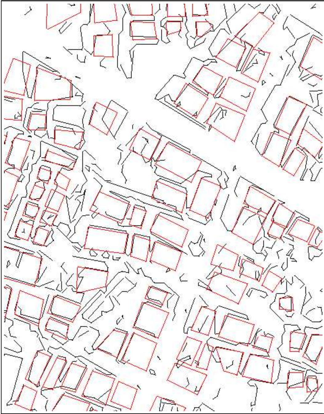
Figure 4.2: The vector building boundaries and the line segments (Vector boundaries in red)
