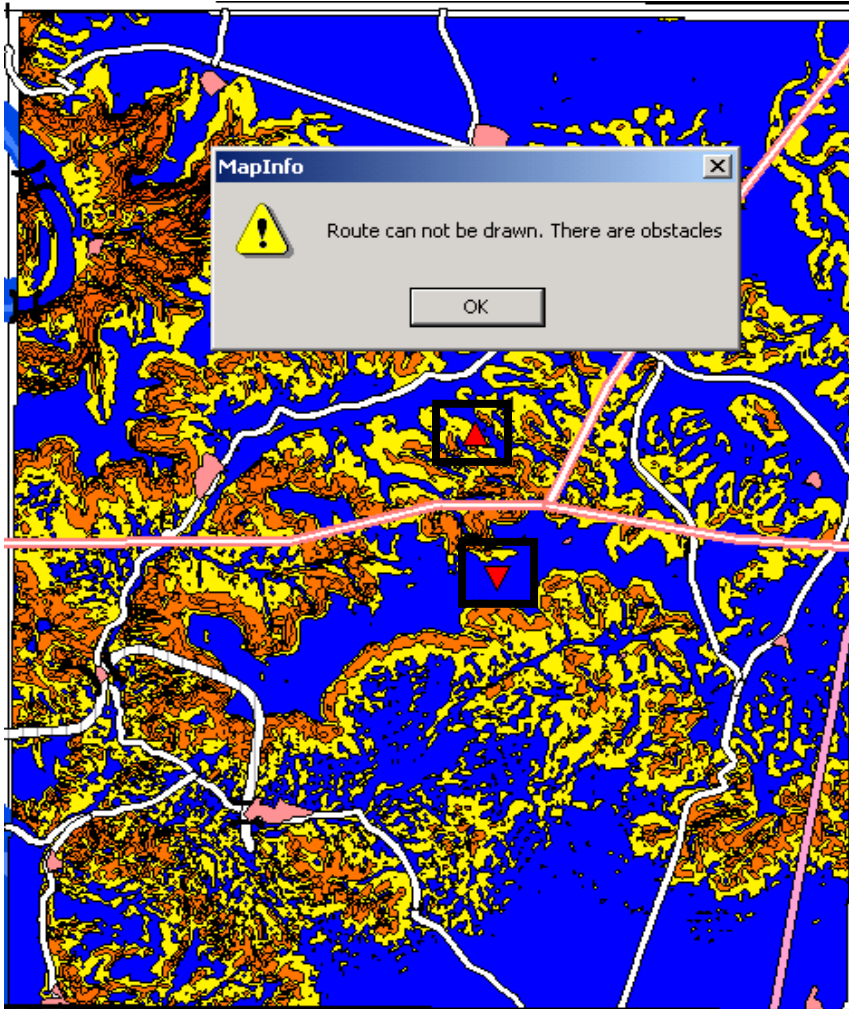
Figure 3.19 Shortest path cannot be found from one side of the motorway to the other
