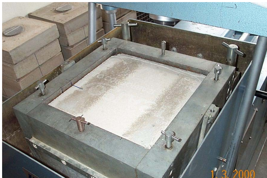
Figure 4.4 Photograph of a test sample built-in shear box
