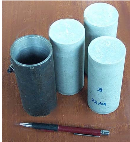
Figure 4.1 Samples prepared for compressive strength tests
