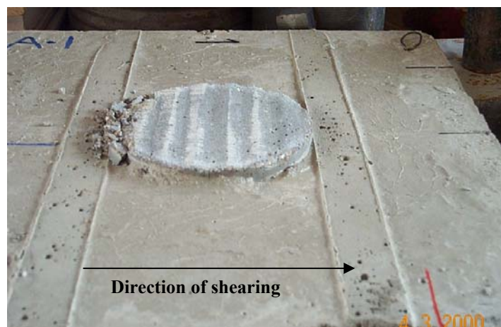
Figure 5.7 Side view of a lower half sample after shear test at 5 kN, fail of the edge also occurred at that normal load level
