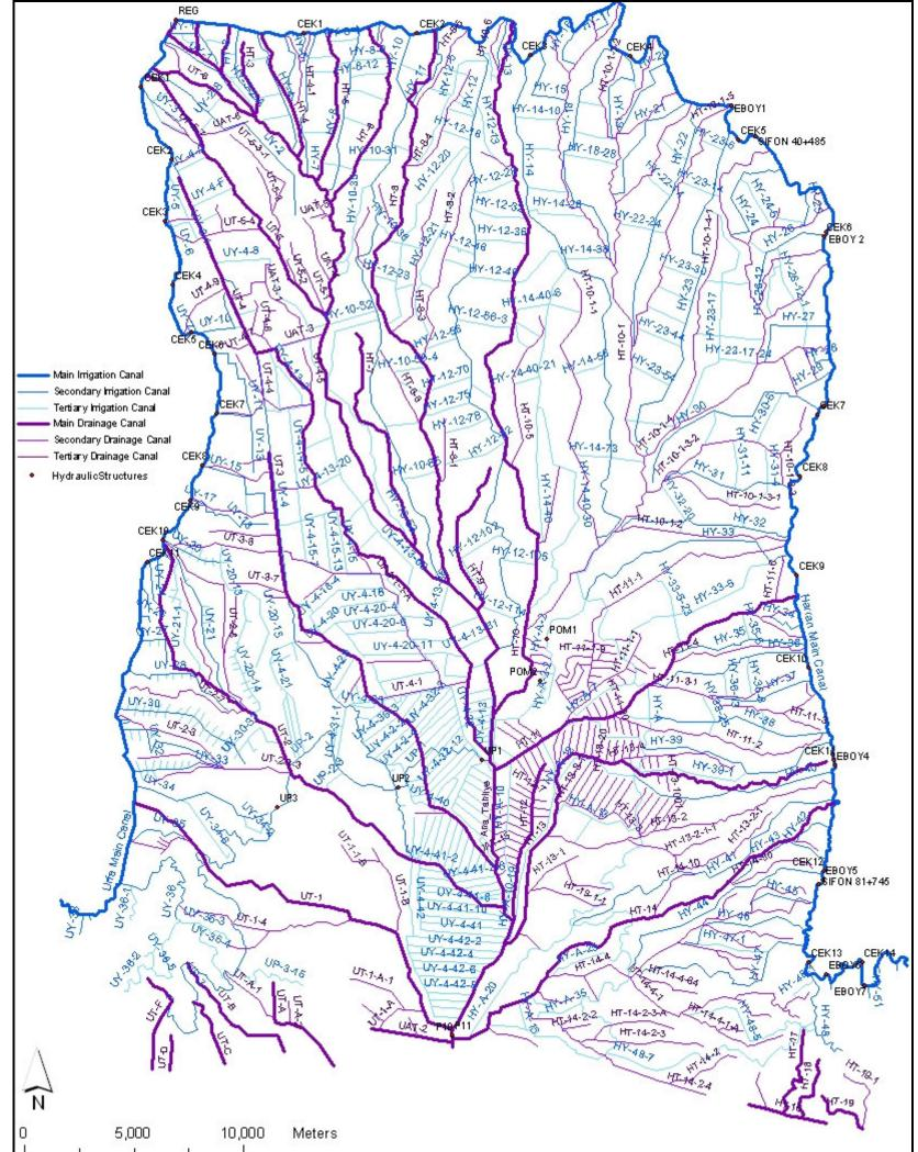
Figure 3.23: Irrigation and Drainage System
