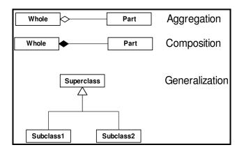
Figure 2.6: Notation for aggregation, composition and generalization
