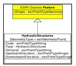
Figure 3.16: Hydraulic Structures Diagram
