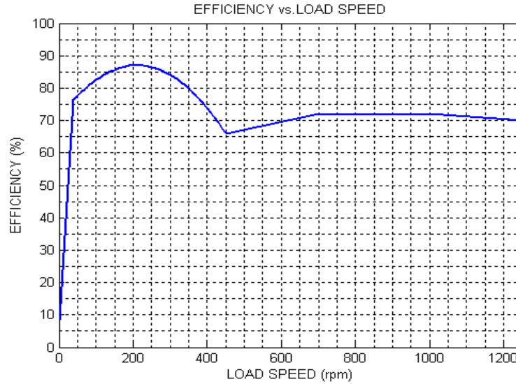
Figure 5.37 Efficiency of 10-pole AF-BLDC
