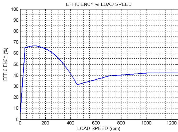
Figure 5 25 Efficiency of 10-pole RF-BLDC
