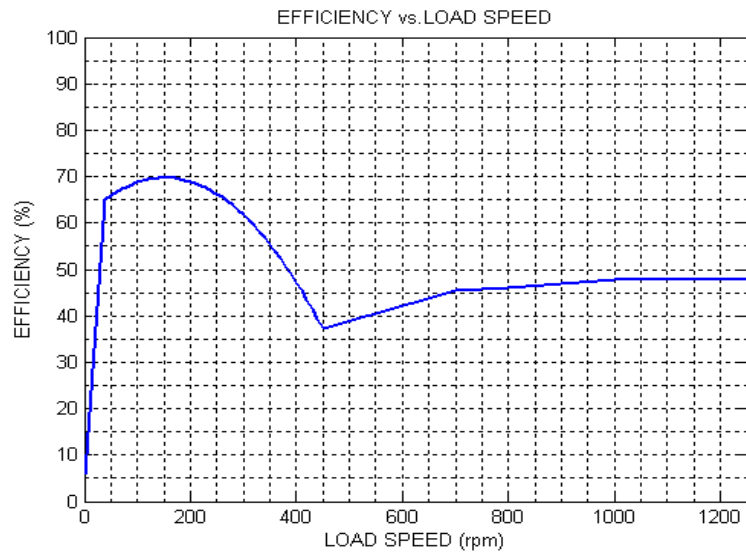
Figure 5 21 Efficiency of 6-pole RF-BLDC
