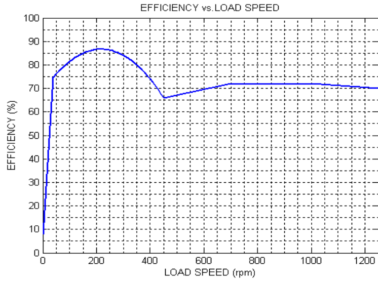
Figure 5 33 Efficiency of 6-pole AF-BLDC
