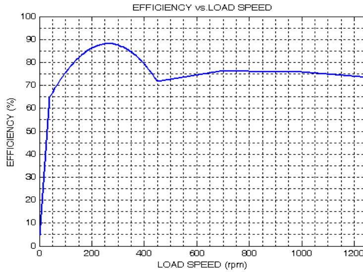
Figure 5 29 Efficiency of 2-pole AF-BLDC
