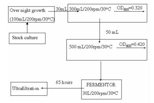
Figure 3.21. Schematic description of pilot scale fermentation studies.
