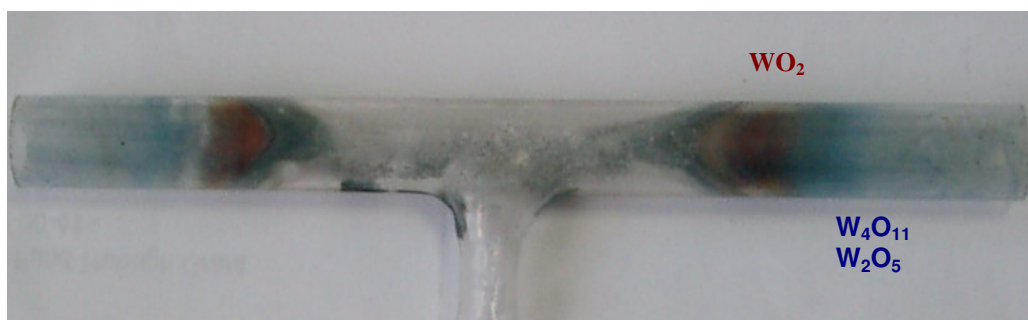
Figure 3.2 The effect of oxidation of W-coil on QTA when H_2 was not used in the carrier gas
