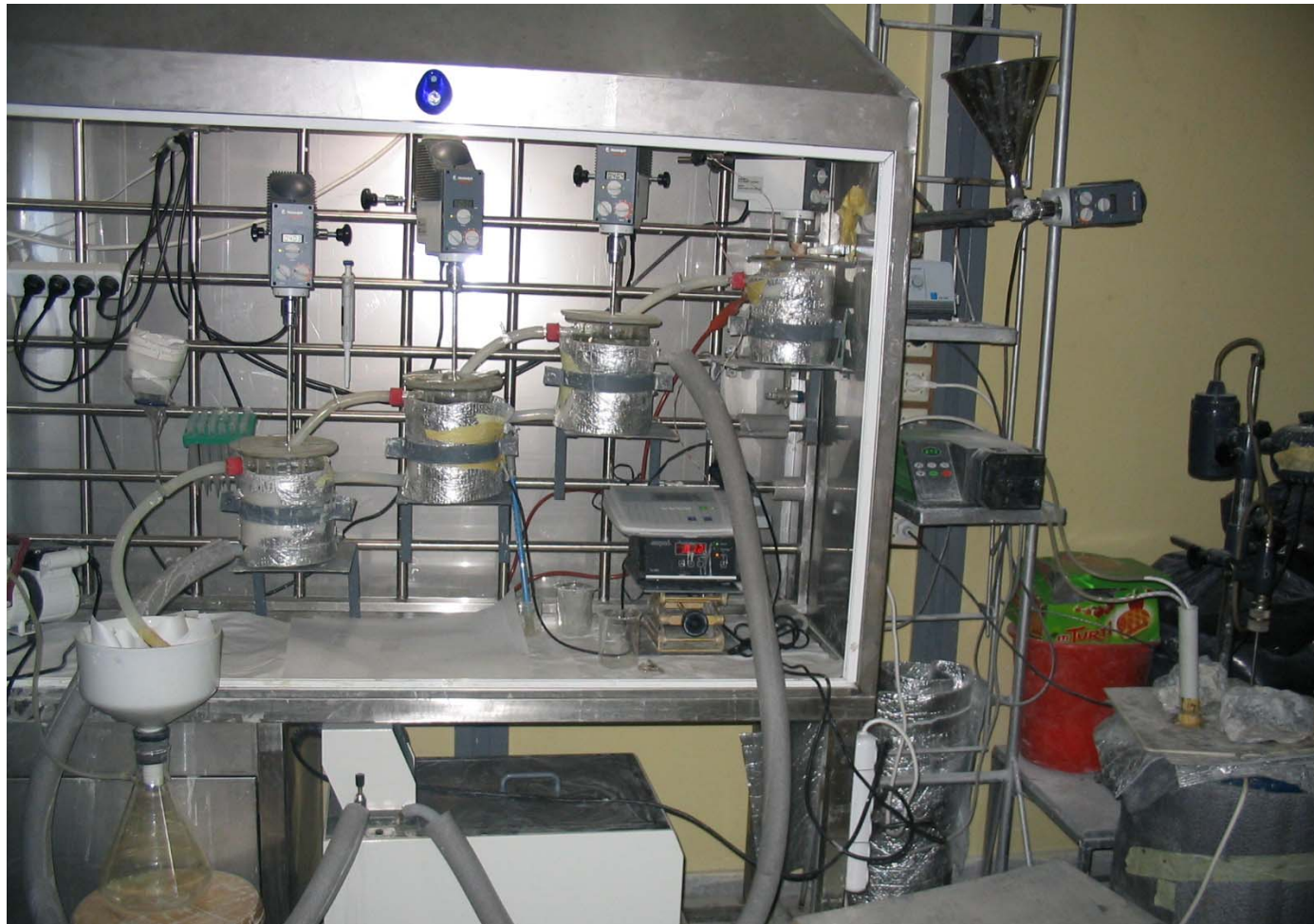
Figure 4.5. Photograph of the set-up used for the continuous flow stirred slurry reactor experiments
