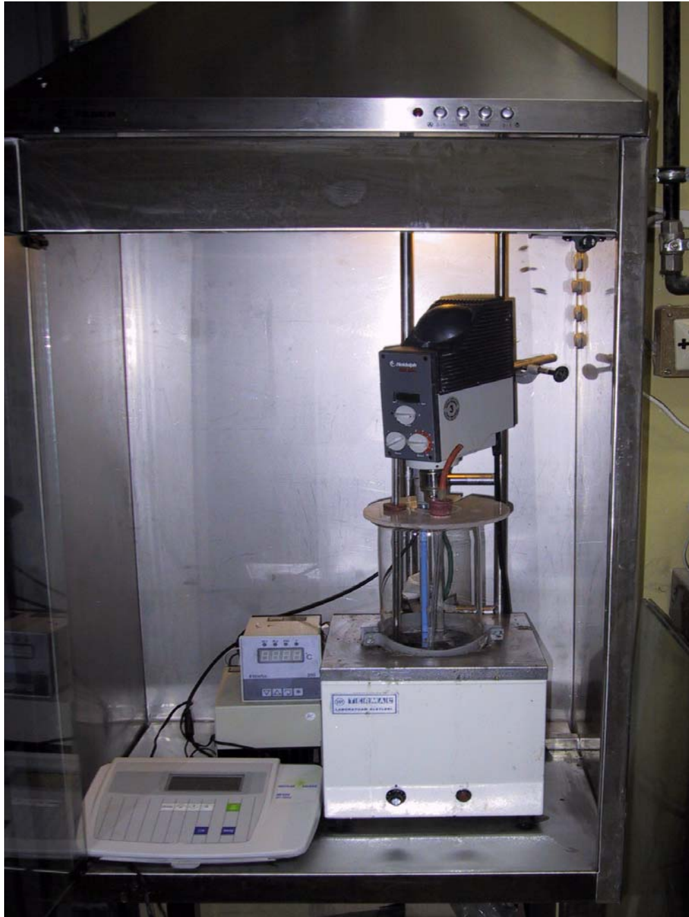
Figure 4.2. Photograph of the set-up used for the batch reactor experiments
