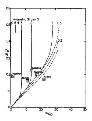
Fig. 4.5: Chart for Determination of Post-Liquefaction Volumetric Strain of Clean Sands (After Tokimatsu and Seed, 1984)
