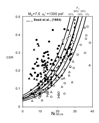
Fig. 2.9(a): Recommended Probabilistic SPT-Based Liquefaction Triggering Correlation (for Mw=7.5) (After Seed et al., 2001)
