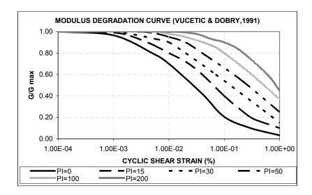
Fig. 3.4: Modulus Reduction Curves for Fine-Grained Soils of Different Plasticity (After Vucetic And Dobry, 1991)
