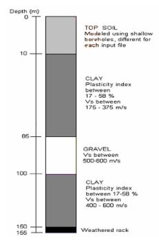
Figure 3.13: Modeled Deep Borehole Logs
