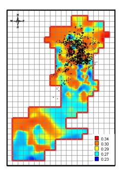
Fig. 3.15b: Peak Ground Acceleration Map Overlaid on Damaged Buildings throughout Adapazarı.
