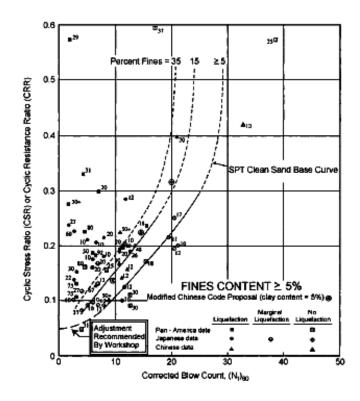
Fig. 2.8: SPT Clean-Sand Base Curve for Magnitude 7.5 Earthquakes with Data from Liquefaction Case Histories (Modified from Seed et al. 1985)
