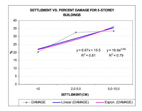
Fig. 5.5: Distribution of the percent number of damaged buildings with liquefaction induced ground settlements.
