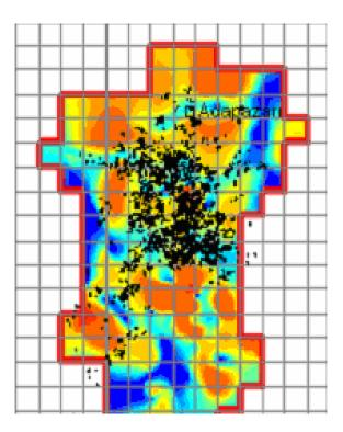
Fig. 4.7(a): Post Liquefaction Volumetric Settlement Map (b): Heavily Damaged Buildings (Black Dots) Overlaid on the Map of Post Liquefaction Volumetric Settlement.
