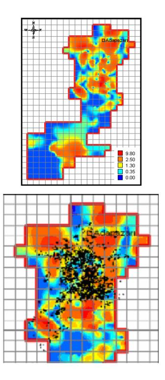
Fig. 4.1 (a): Liquefaction Severity Index Map (b): Damaged Buildings (Black Dots) Overlaid on the Map of Liquefaction Severity Index.
