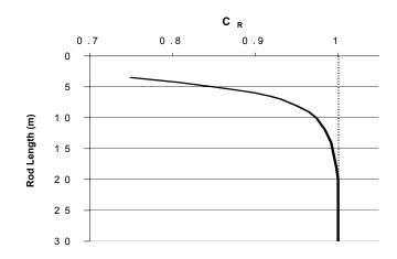
Fig. 2.10: Recommended CR Values (rod length from point of hammer impact to tip of sampler). (After Seed et al., 2001)
