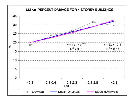
Fig. 5.4: Distribution of the Cumulative Number of Damaged Buildings with Liquefaction Severity Index.
