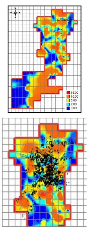
Fig. 4.3(a): Thickness of the Potentially Liquefiable Layer Map (b): Damaged Buildings (Black Dots) Overlaid on the Map of Thickness of the Potentially Liquefiable Layer
