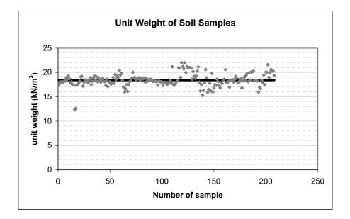
Fig. 3.3: The Scatter of the Unit Weight of Soil Samples Tested in the Laboratory
