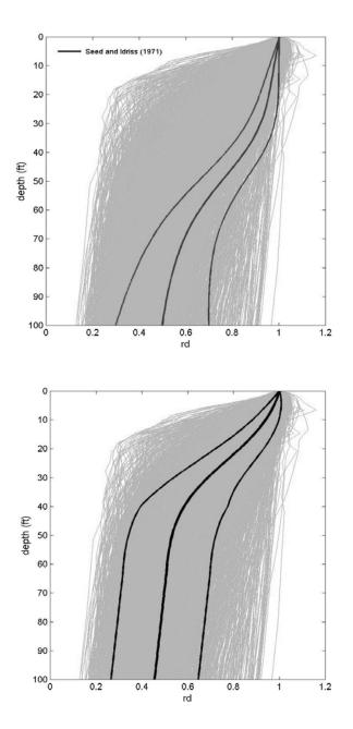
Fig. 2.7: Rd Results from Response Analyses Superimposed with Heavier Lines Showing (a) the Earlier Recommendations of Seed and Idriss (1971), and (b) the Mean and + 1 Standard Deviation Values (After Seed et al., 2001)
