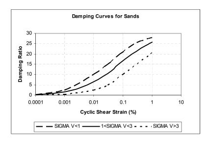
Fig. 3.7: Damping Curves for Sands (After Seed And Idriss, 1970)
