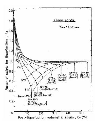
Fig. 4.6: Chart for Determination of Post-Liquefaction Volumetric Strain of Clean Sands as a Function of Factor of Safety (After Ishihara, 1996).
