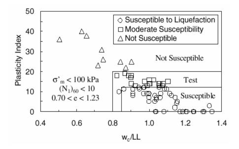
Fig. 2.4: Criteria for the Evaluation of the Liquefaction Susceptibility of Fine-grained Soils at Low Confining Stresses. (After Bray et al., 2003)
