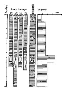
Figure 3.12: Second Set Of Borehole Logs (Deep)
