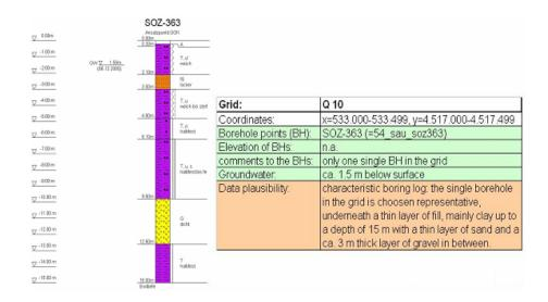
Figure 3.11: Representative Soil Profile For Grid No: Q10
