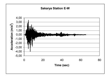
Fig. 3.14: The Acceleration vs. Time (East – West) Plot Recorded At Sakarya Strong Ground Motion Station
