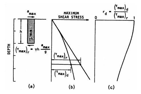
Fig. 2.5: Illustration of Simplified Procedure (After Seed and Idriss, 1971)
