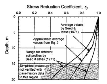
Fig. 2.6: Rd versus Depth Curves Developed by Seed and Idriss (1971) with Added Mean-Value Lines Plotted (After Youd et al., 2001)
