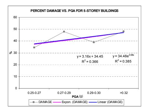
Fig. 5.2(b): Distribution of the Percentage of Damaged Buildings with PGA for 5-Storey Buildings
