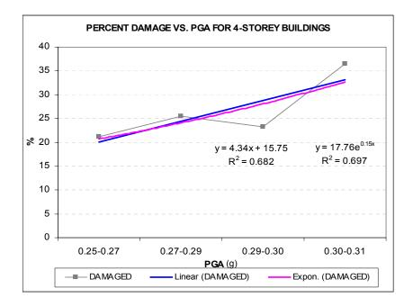
Fig. 5.2(a): Distribution of the Percentage of Damaged Buildings with PGA for 4-Storey Buildings
