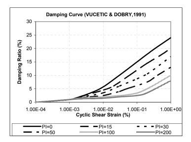
Fig. 3.6: Damping Curves for Fine-Grained Soils of Different Plasticity (After Vucetic And Dobry, 1991)
