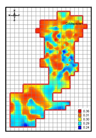
Fig. 3.16: Distribution of Spectral Acceleration for T=0.1 second throughout Adapazarı.
