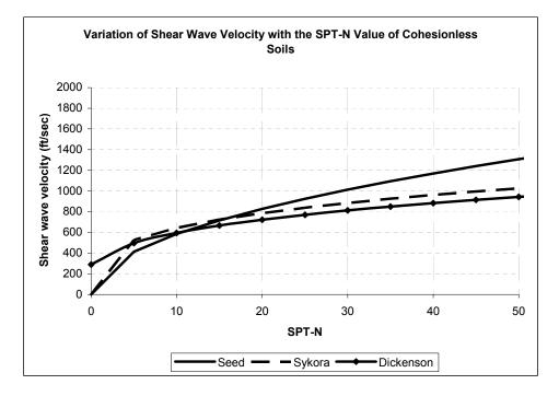
Fig. 3.2: The Correlations Used in Converting SPT-N Values to Shear Wave Velocities
