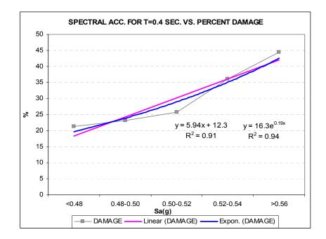
Fig. 5.3(a): Distribution of the Percentage of Damaged Buildings with Spectral Acceleration Corresponds to T= 0.4 Sec for 4-Storey Buildings.
