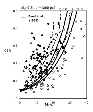
Fig. 2.9(b): Recommended "Deterministic" SPT-Based Liquefaction Triggering Correlation (for Mw=7.5), with Adjustments for Fines Content (After Seed et al. 2001)
