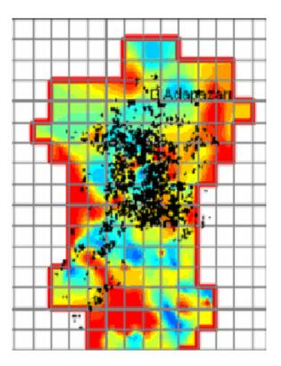
Fig. 4.4(a): Representative Depth to the Potentially Liquefiable Layer Map(b): Heavily Damaged Buildings (Black Dots) Overlaid on the Map ofRepresentative Depth to the Potentially Liquefiable Layer.
