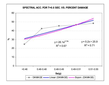
Fig. 5.3(b): Distribution of the Percentage of Damaged Buildings with Spectral Acceleration Corresponds to T= 0.5 Sec for 5-Storey Buildings.
