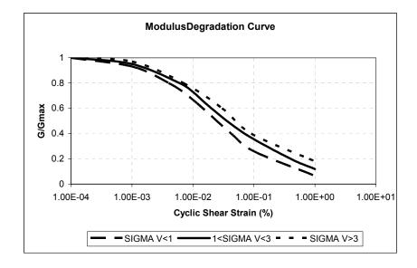
Fig. 3.5: Modulus Reduction Curves for Sands (After Seed And Idriss, 1970)
