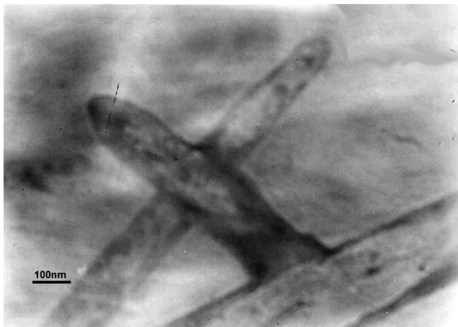
Figure 4.24 A higher magnification image of the three nanotubes in figure 4.23. Magnification x66k.
