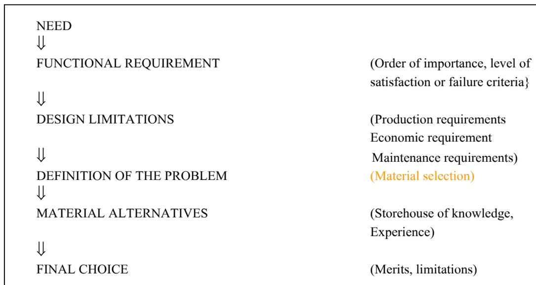
**Figure 3.3** A simple flow diagram of design thinking for material selection (Esin, 1980, 151).
