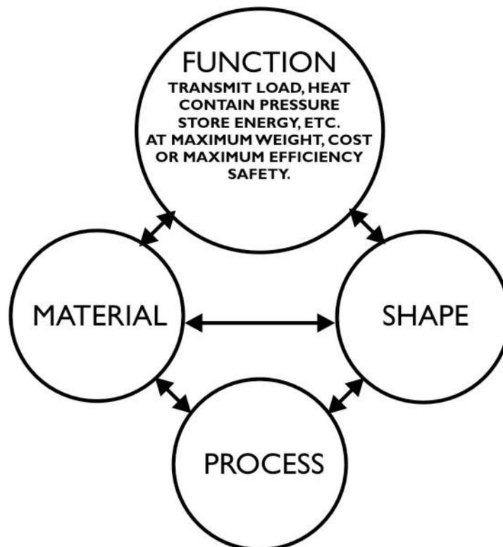
**Figure 3.4** The interaction between function, material, process and shape (Ashby, 1992, 10).
