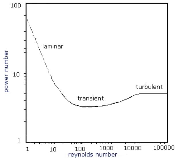
**Figure 4.11** Correlation between the power number and the Reynolds number for a bioreactor system with one-six bladed Rushton turbine impeller and baffles.
