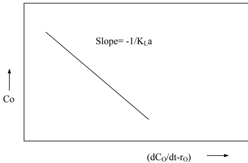
**Figure 2.4** Evaluating  $K_L a$  using the Dynamic Method
