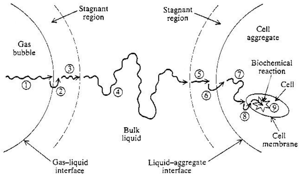
**Figure 2.2** Overview of steps in the overall mass transfer of oxygen from a gas bubble to the reaction site inside the individual cells.
