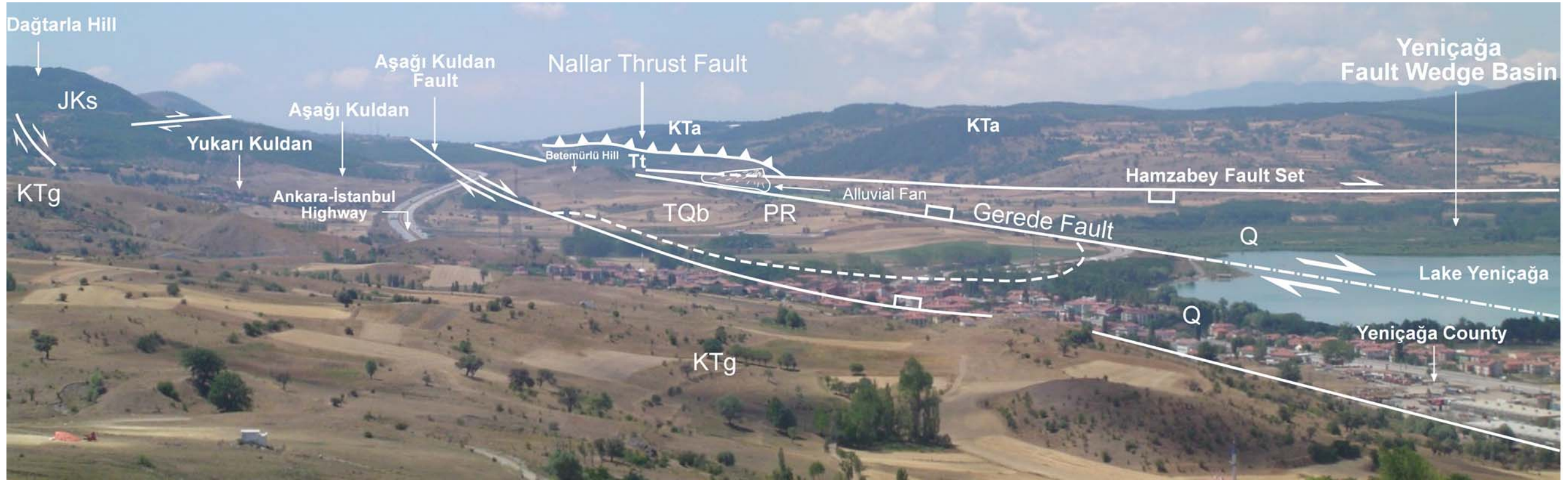
Figure 40. General view of the western half of the Yeniçağa fault-wedge basin and its margin – bounding faults. JKs: Upper Jurassic-Lower Cretaceous Soğukçam Limestone, KTa: Upper Cretaceous ophiolitic mélange ( the “Arkotdağ Formation”), KTg: Upper Cretaceous – Upper Miocene Galatean Arc Complex, Tt: Lower-Middle Eocene Taşlık Formation, TQb: Plio-Quaternary Betemürlü formation, Q: Quaternary Alluvial sediments, PR: Pressure Ridge (Location ~ 2 km E of Yukari Kuldan Village, view from SE to NW)
