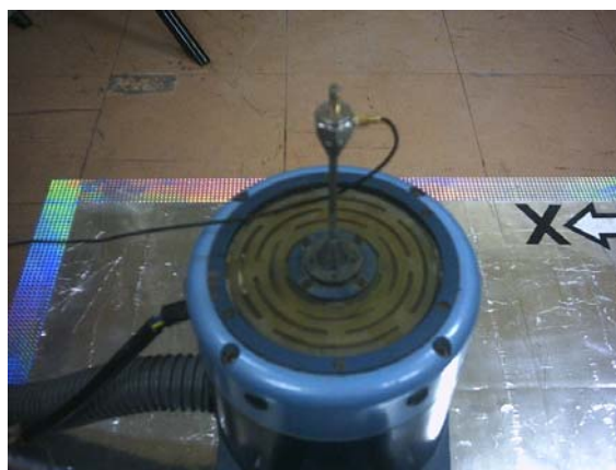
Figure 4.42 Force Transducer Assembled onto the Stinger
