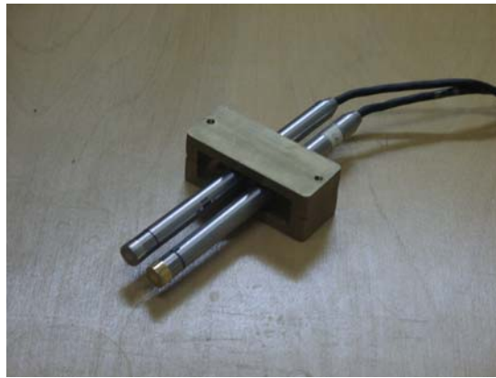
Fig 3.6 An Intensity Probe Having a Side-By-Side Configuration
