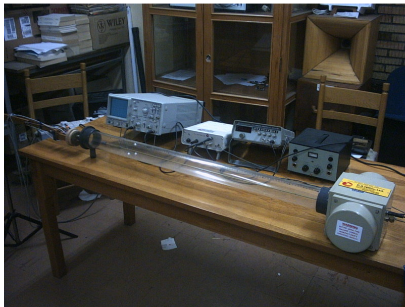
Figure 4.57 Phase Mismatch Error Measurement Set-Up
