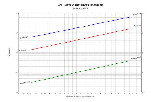
Figure B.15– Effect of Volume on Reserves Estimate for Field B
