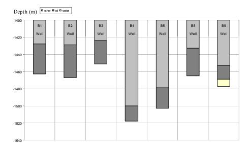
Figure B.5-Log Analysis Depth Plot for Field B
