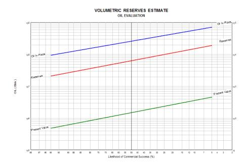
Figure B.11-Effect of Saturation on Reserves Estimate for Field A
