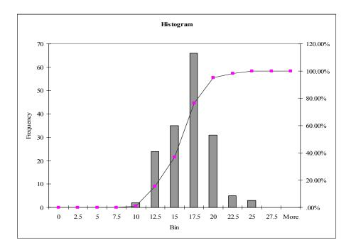
Figure B.6 - Porosity Distribution Histogram for Field B
