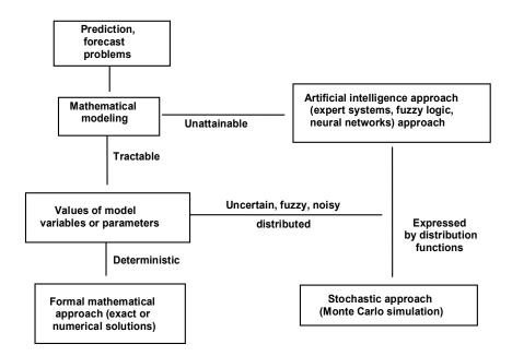
Figure 2.1- How Prediction Tools are Implemented
