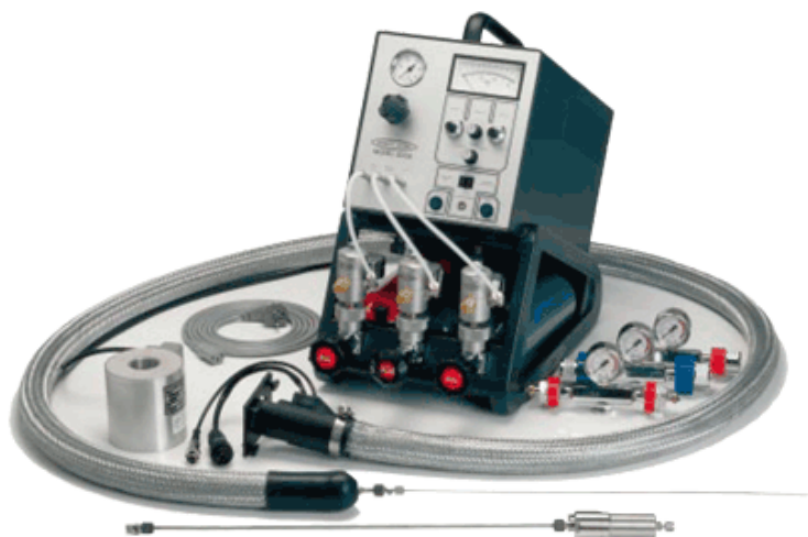
Figure 3.4 A general photograph of Total VOC Analyzer
