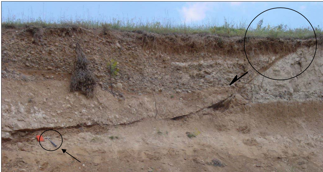
Figure 4.17. Close-up view of the Fault-24. Note that it cuts through the soil (hammer at left of the photo for scale, 33-cm long).
