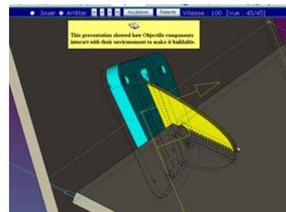
3-7. Screen captures from the software “Objectile.” The capture at right side shows how a connection is configured to serve for different parts come together. (Source: [WWW, Internet], Objectile website, Address: http://www.objectile.org , [Last Accessed: 12.06.2004])
