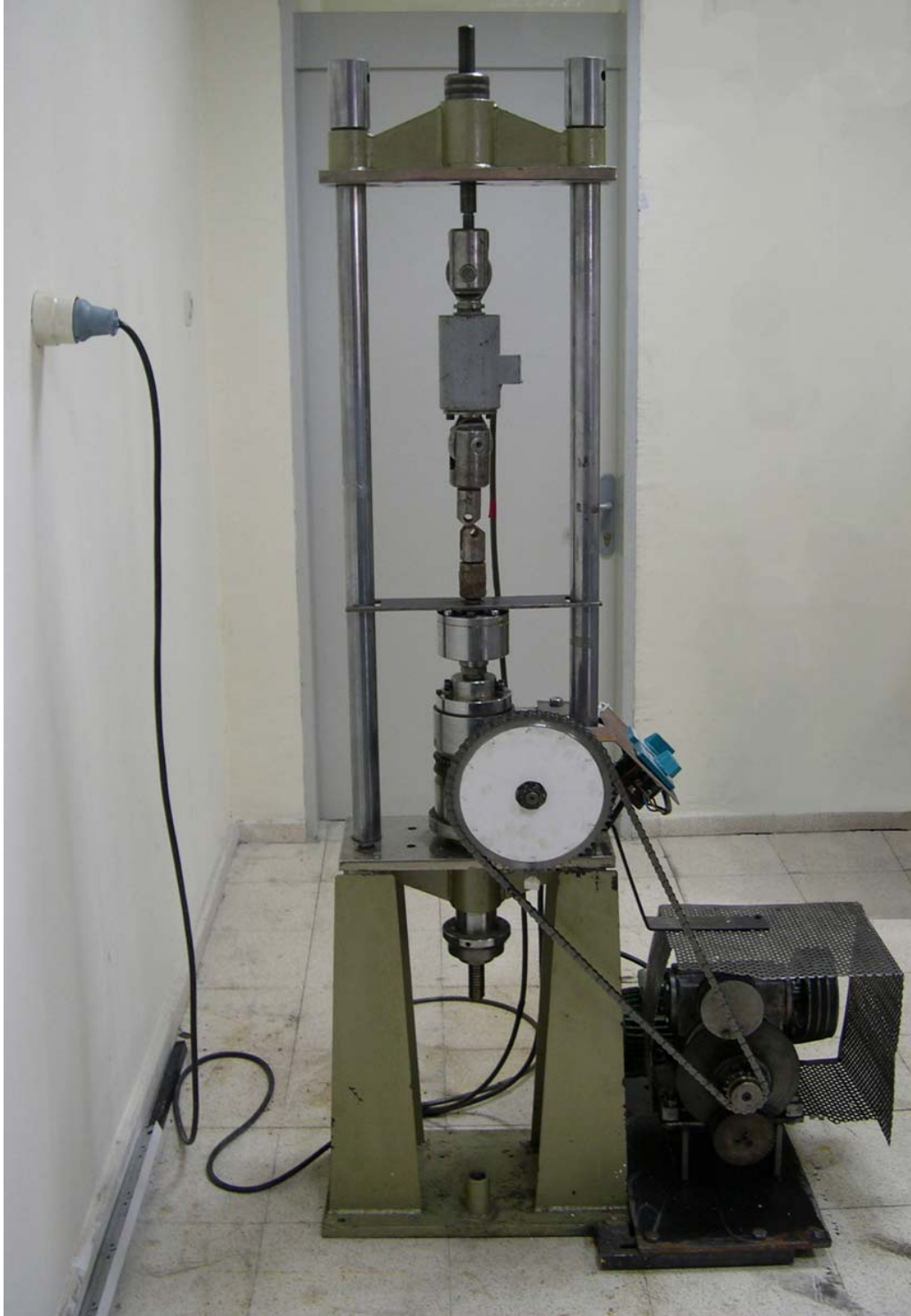
Figure 3-8 Photograph of Constant Extension Rate Testing system.
